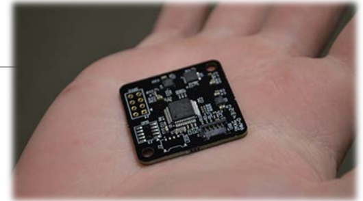
Gyroscope in Oculus Rift DK1
