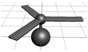
The figure above shows a simple helicopter model. It contains a body, a vertical axis, a top sphere (to hold the main propeller) and three rotor blades. The grid in the background indicates the location of the x-y plane. The z axis points up.
