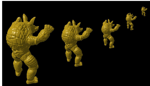
Size dependent mesh reduction (Data: Stanford Armadillo)
