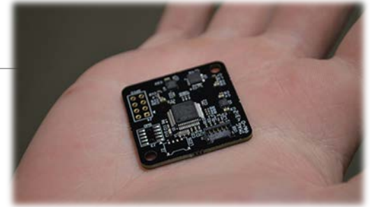
Gyroscope in Oculus Rift DK1
