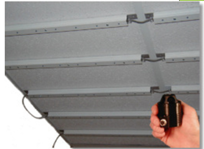
HiBall beacon array
