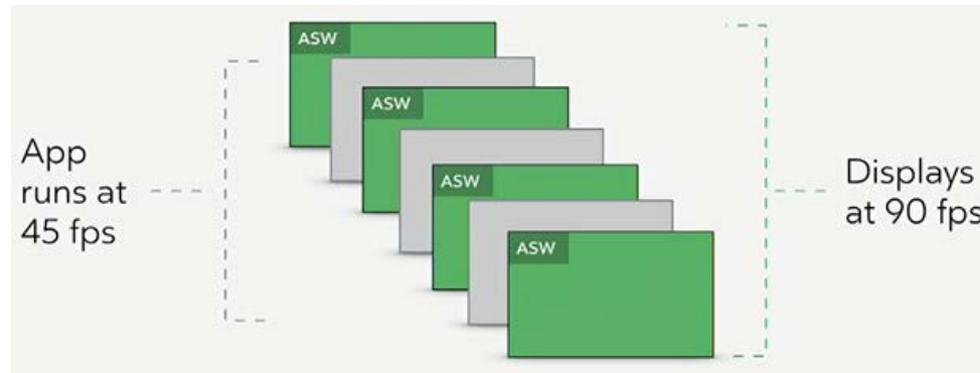
When an application fails to render frames at 90Hz, the Rift driver drops the application down to 45Hz with ASW providing each intermediate frame.
