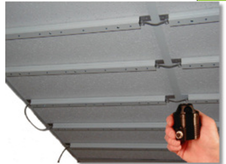
HiBall beacon array
