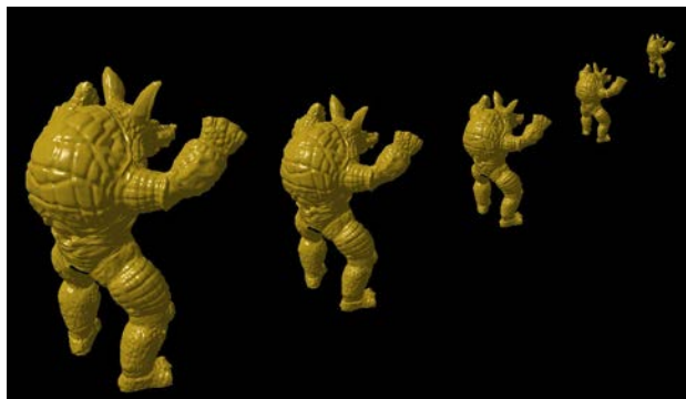
Size dependent mesh reduction (Data: Stanford Armadillo)
