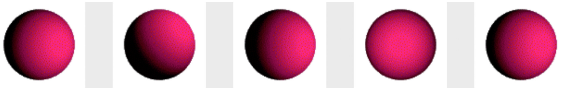
Lambertian (diffuse) sphere under different lighting directions
