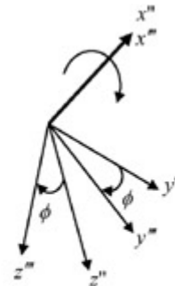
3 rd , the body frame rolls CW an angle \phi about the x'' -axis
