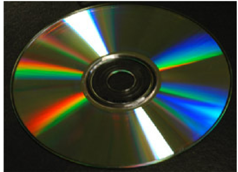
Surface of a CD shows diffraction grating
