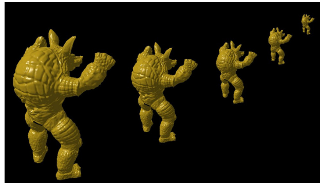
Size dependent mesh reduction (Data: Stanford Armadillo)
